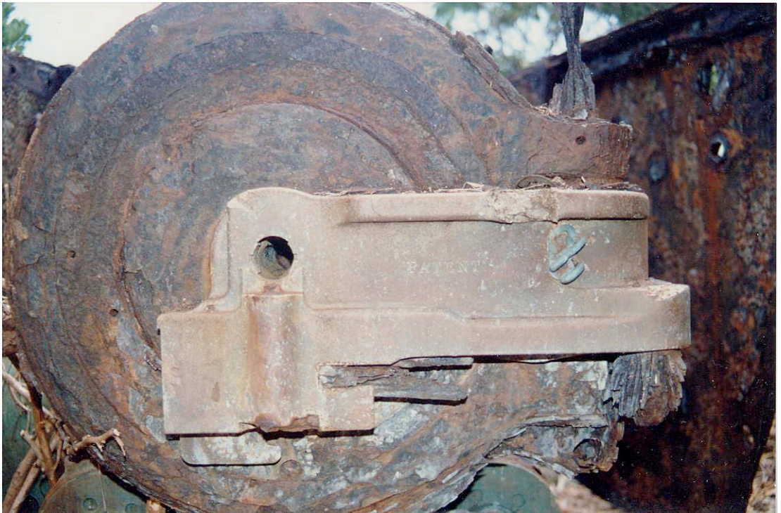
Figure 5. Breechblock of a Elswick Ordnance Company 6-inch gun on Taroa I., Maloelap Atoll
