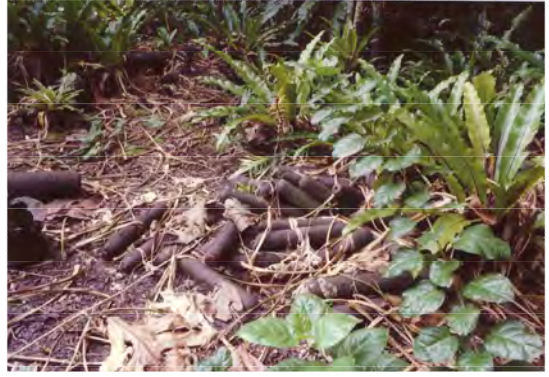
Fig. 40. Compressed air cylinders for use in Mitsubishi A6M 'Zero' fighter aircraft, piled up in a corner of the aircraft hangar or Mile Airbase. While perfectly harmless, uninitiated visitors might mistake these for unexploded ammunition.. (Mile I., Mile Atoll, RMI).
