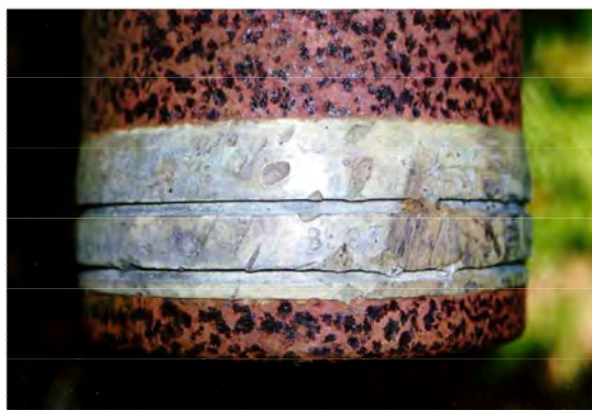
Fig. 34. Impact damage to the bourrelet ring of the 150mm shell shown in Fig. 41. (Madelonimwb Harbour, Temwen I., Pohnpei, FSM)
