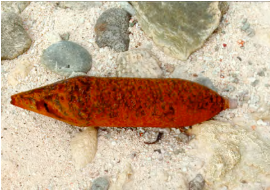
Fig. 17. Unexploded aerial bomb. Note that the tail fins of the bomb (at left) are missing, while the fuse is still undamaged. (Wotje I., Wotje Atoll, RMI).
